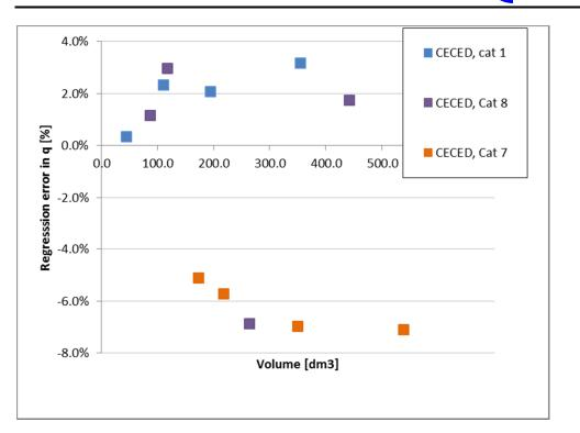
This shows that for such products the reference curve predicts 6 to 7 % lower consumption values than the model, or in other words, such products need to be 7 % more efficient to obtain the same efficiency class. The opposite is the case for products having a higher fresh food fraction than 73 %.
