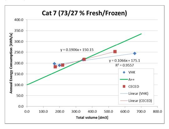
Compared to the VHK data the curve is now more steep, bit still significantly flatter than the current A++ curve, so larger appliances are penalised compared to today.
