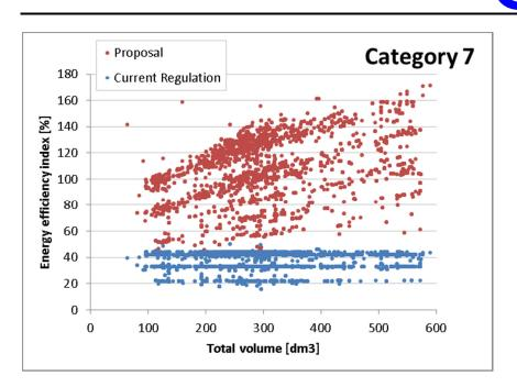
The final result on category 7 show a steep increase as function of the volume. A limit at index 100 would cancel out all current  $A_{++}$  appliances with a total volume larger than app. 250 litre (uncorrected for the global standard).
