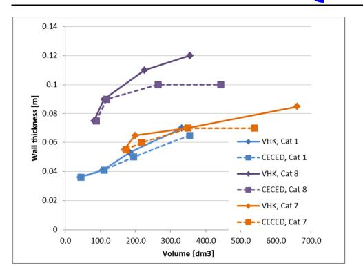
The chart above shows the wall thicknesses as applied in the model, it needs mentioning that the values given here are typical for free standing appliances but difficult to meet for built-in.
