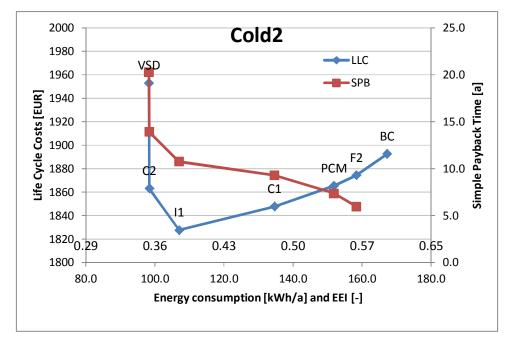
The minimum LCC is found here around an index of 0.40 instead of 0.31 in the report. The difference is mainly because of the index calculation of the base case. and by the fact that option D2 is not seen as an option. The saving is approximately 36 % in energy.
