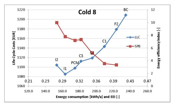
The final conclusion is different from the one in the report where the minimum value (LLCC) is around 1050 EUR at an index of 0.23 while here the minimum is 1085 EUR at index 0.29 with a saving of 30 % in energy.
