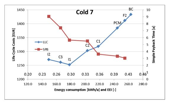
The minimum LCC is found here at an EEI of approximately 0.3 whereas the report finds the minimum around 0.23. This difference is partly caused by the difference in the model, but also for a part due to a possible mistake in the EEI calculation in the report. The energy saving is app. 32 %.
