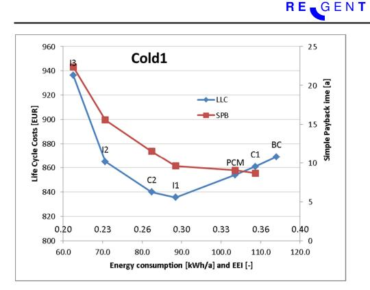
The final conclusion is not very different from the one in the report, the minimum value (LLCC) is around 830 EUR resulting in an index around 0.3 and a saving of app. 25 % in energy. Note that payback times are quite high.
